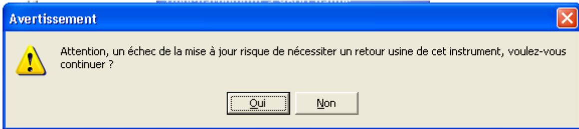
**Never interrupt the procedure while downloading.** If a full update is interrupted, the device must be sent back to factory
